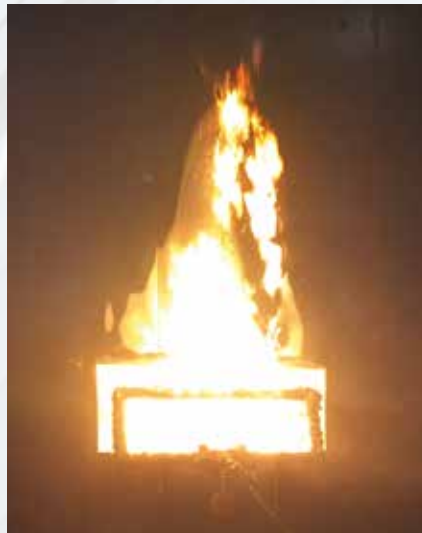
During the test a fire source simulates fire coming out of a window opening.
