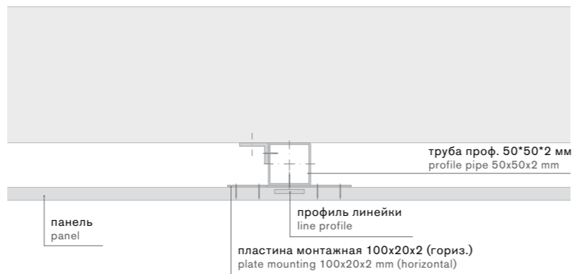
Узел крепления стыка двух панелей через линейку, стык 10 мм. Fixing joint between two panels through the line, the joint is 10 mm.
