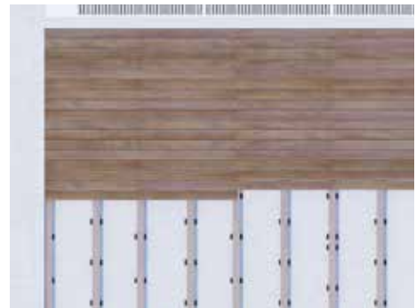
picture A - correct installation: the installation is made along rows, with a staggered fashion.
