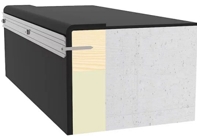
Installation on a concrete upstand
